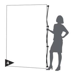
Adjust leveling knobs for desired angle. OneFabric<sup>™</sup> display can now be moved easily into position.
