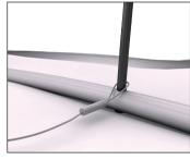
7. Place the black vertical shafts in the bottom ring.
