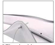
6.Thred cable support through eyelet.
