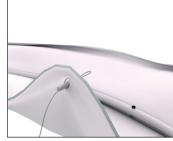
6.Thread cable support through eyelet.
